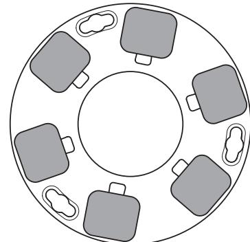
By changing the way the diamonds are set-up on the diamond holder discs, an operator can significantly effect the performance of the machine and therefore, the finished product.
