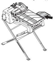
If the side table is not in level with the conveyor cart it may need adjustment. Adjust using the screws.
