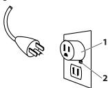
The temporary adapter should be used only until a properly grounded outlet can be installed by a qualified electrician.
