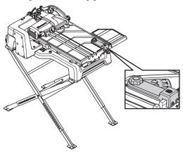
• Assemble the water recovery tray. Make sure that the plastic hook grips the metal bar under the cart.
