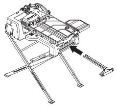
• Connect the water hose (2) and the water pump (1) to the connectors on the frame.
