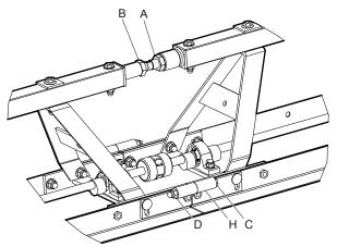
8. The nuts (A) will be tightened after the crown adjustment is done.
