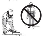
Place the chain saw on the ground and hold the rear handle down with your right foot. Grasp the front handle firmly using your left hand. Make sure the chain saw is steady and the chain is not touching the ground or other objects. Then grasp the starter handle with your right hand and pull the starter cord. Never twist the starter cord around your hand.
