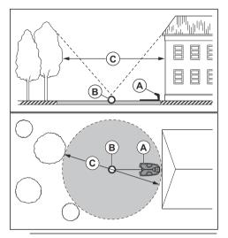
**Note:** Short reversing distance decreases the risk of track marks. A long reversing distance can be necessary to have good satellite signals at the docking point.
