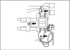
9. Disconnect the batteries connection from the main circuit board.
