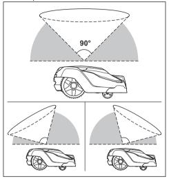
**Note:** Objects that are less than 1 m / 3.3 ft. in height (A) does not impede the satellite signals.
