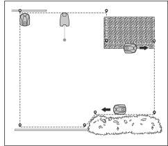
Add a waypoint to make the product cut the grass at the edge between the lawn and the stone path. Make sure that you straddel the edge of the lawn and the stone path when you add a waypoint. The product can straddel the edge if the height of the stone path is maximum 1 cm / 0.4 in. in relation to the lawn.
