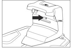
If the indicator LED lamp does not have a green light, do a check of the installation. Refer to *To* install the charging station on page 16 and LED indicator lamp on the charging station on page 38.
