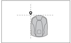
**Note:** The position of the waypoint when you install a transport path or a path to a maintenance point is in the middle of the product between the drive wheels.
