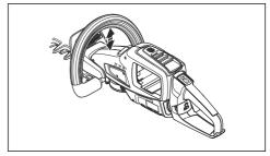
3. To apply full speed, push the power trigger fully.
