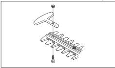
Assemble the screw and the nut to the cutting unit and tighten to 8 Nm.
