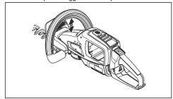
3. Push the power trigger up and apply full power.
